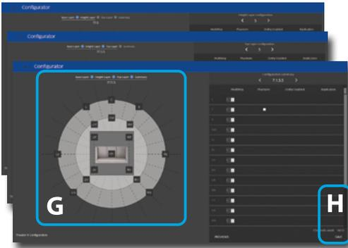
**G.** At the end, a summary of the Speakers Configuration is shown. A four digits description is given following this order: "Base Layer . LFE . Height Layer . Top Layer".
