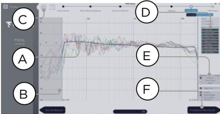
Once all measurements are complete, you can visualize measurements of each speaker. You can customize the target curve for each speaker by (A) limiting the correction window and (B) dragging anchor points on the target curve to desired locations. By default a target curve is proposed offering a typical cinema curve. It is possible to save or load target curve through menu (C). Good target curve design is beyond the scope of this document, but there are some key points to remember.
