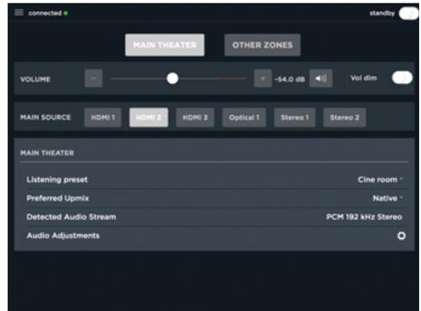
Touch one of the 5 icons at the bottom of the screen to access features found in the web UI remote including the Main Theater control as shown below.
