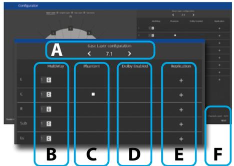
A. Choose using the left and right arrows which speaker combination you expect for the layer amongst predefined options populated automatically depending on the channels decoding capability of the ISP version.
